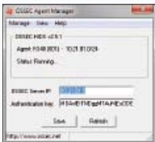
Figure 4: In contrast to syslog integration, the Windows agent uses a secure encrypted connection to transfer its data by default.
